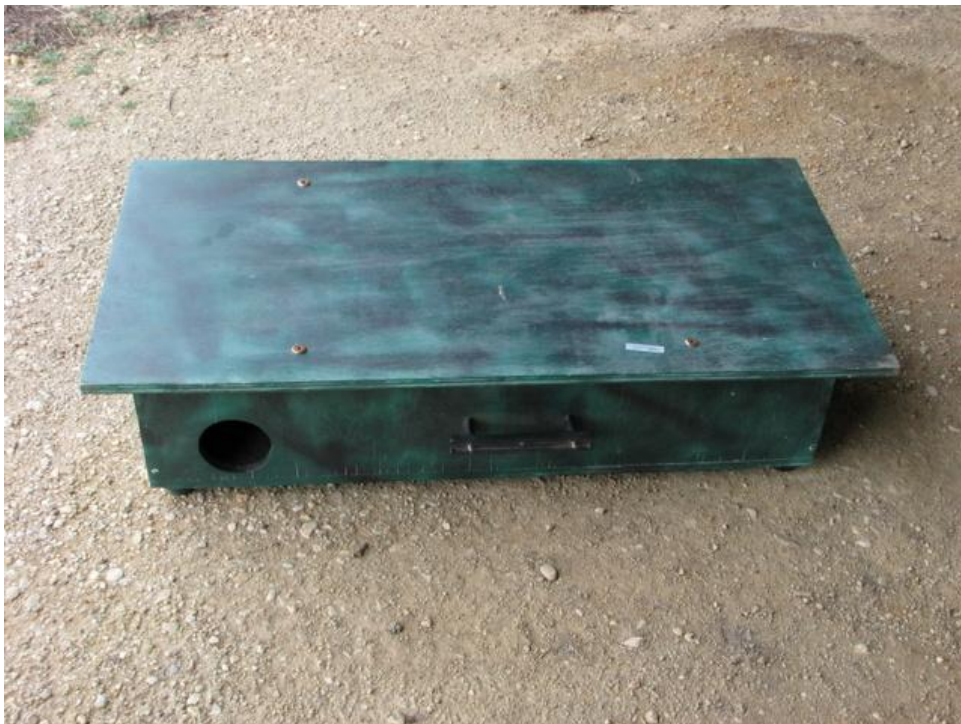
Figure 1: First version of the camera box assembled for use. Note carry handle on side and access hole near one end. There is an identical access hole on the opposite side.
